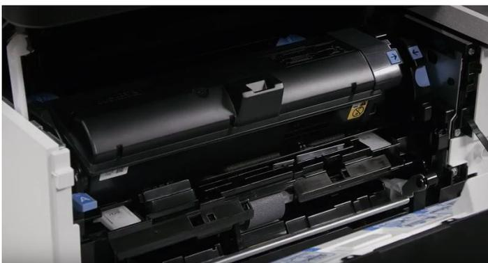
Procedures for replacing toner are easy. Although it can't be replaced while the unit is running, the cartridge is accessible from the front and lifts out easily after a blue lever on the left has been released.
