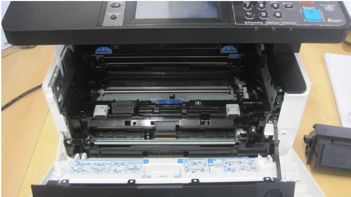
Misfeed access is either at the front (shown above) or at the rear of the device. If accessed at the front, the drum unit needs to be removed, but the surface of the drum is not exposed to any risk of damage during removal.
