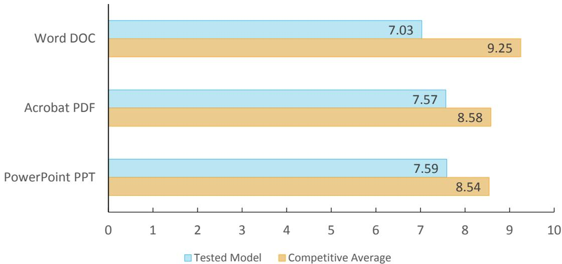
First-print time indicates the time it took to process, image and deliver a single-page document to the output tray. The unit's print speeds were tested at the default 600 dpi using the PCL driver.
