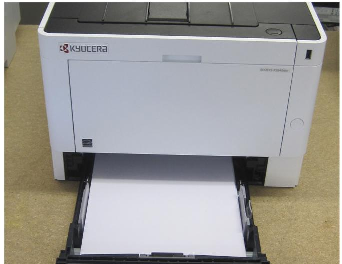
BLI technicians noted that loading paper trays is easy, with sliding paper guides, which move in sync. As is typical of models in this class, paper sizes must be confirmed on the LCD screen.
