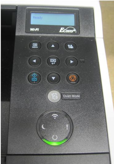
The KYOCERA ECOSYS P2040dw has a very simple, intuitive control panel design with a small LCD display, and up/down and left/right keys for menu navigation.
