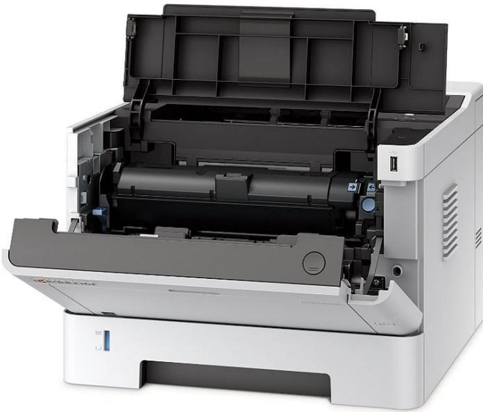
Procedures for replacing toner are easy. Although it can't be replaced while the unit is running, the cartridge is accessible from the front and lifts out easily, after a blue lever on the left has been released.
