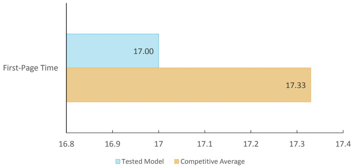
Device sits idle overnight; a single-page black Word document is sent to the device; first-print time indicates the time it took to warm up, process, image and deliver the test document to the output tray.
