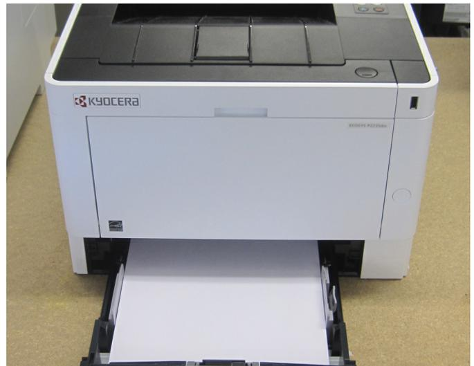
Misfeed access is either at the front (shown above) or at the rear of the device. If accessed at the front, the drum unit needs to be removed, but the surface of the drum is not exposed to any risk of damage during removal.
