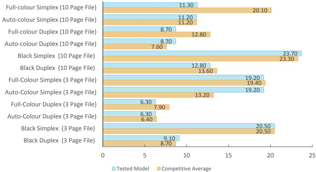
Print speed is tested using a 3-page and a 10-page colour document. BLI obtains the overall speed by averaging the tested speed for each run length (1, 5, 10 and 20 sets). The unit was tested using PCL 6.
