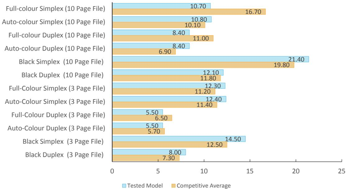
Single-set speed is tested using 3-page and 10-page mixed-colour and black documents. The unit was tested using the PCL driver.
