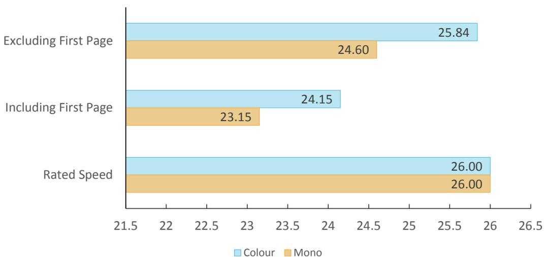
Print speed is tested using BLI's Monochrome Test Original with 6% page coverage. The test page is printed in a quantity equal to double the vendor's rated print speed for the device in each mode tested (e.g., if the vendor's rated print speed is 20 ppm, 40 pages are printed). The unit's print speeds were tested using the PCL 6 driver.
