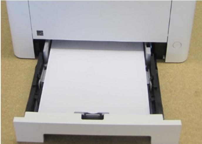
Loading media is straightforward, as is adjusting the tray for different size paper; width paper guides slide in sync.
