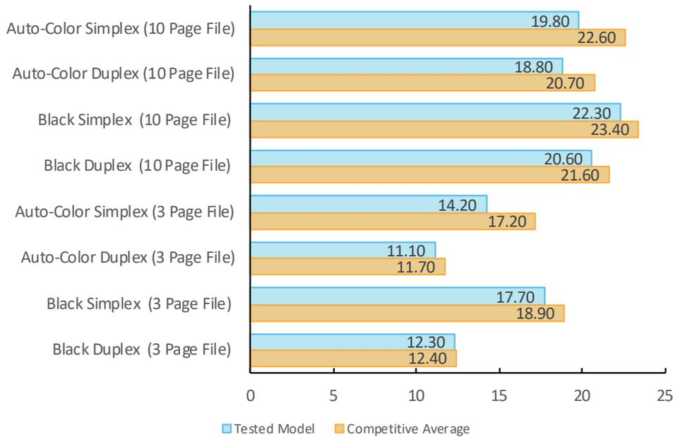
Speed is tested using Buyers Lab's proprietary 3-page and 10-page testing documents. Buyers Lab obtains the overall speed by averaging the tested speed for each run length (1, 5 and 10 sets). The unit was tested using the PCL driver.
