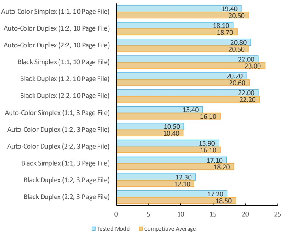
Copy speed is tested using 3-page and 10-page mixed-color and black documents. Buyers Lab obtains the overall speed by averaging the tested speed for each run length (1, 5 and 10 sets).
