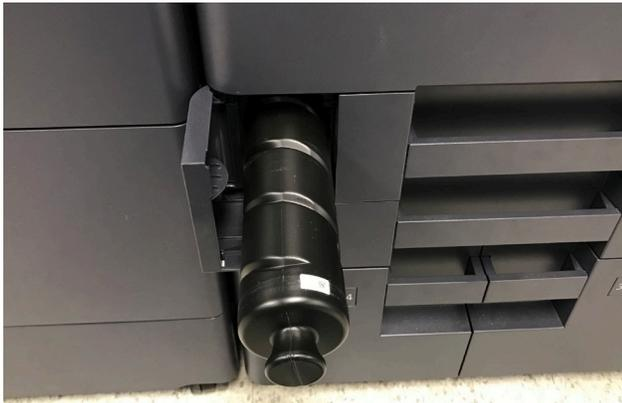
The black toner bottle can be reused as a waste toner bottle. Simply remove the black toner bottle when it is empty, rotate the bottle, and insert the bottle into the waste toner slot.
