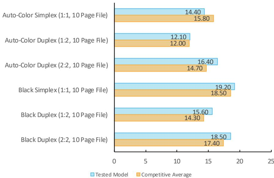
Single-set copy speed is tested using 3-page and 10-page mixed-color and black documents. Timing begins as the start button is pressed, pages are scanned through the document feeder and timing ends when the last page of a single-set of the document exits the device.
