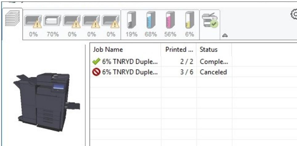
When the user sends a print job a pop up box appears showing all the paper trays and amounts of paper available in each drawer in percent increments, toner remaining in percent increments, and jobs in the print queue. Print job completion and deletion are supported. However, if the user closes out the pop up box during the print process, print job completion and/or deletion will not reappear.
