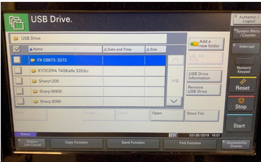
The print from USB menu is automatically populated, with support for PDF, JPEG, and TIFF formats. Users can also change settings for quantity, simplex/duplex, color/mono, and paper size and source. Users can also navigate and print from sub-folders. However, file preview did not function.
