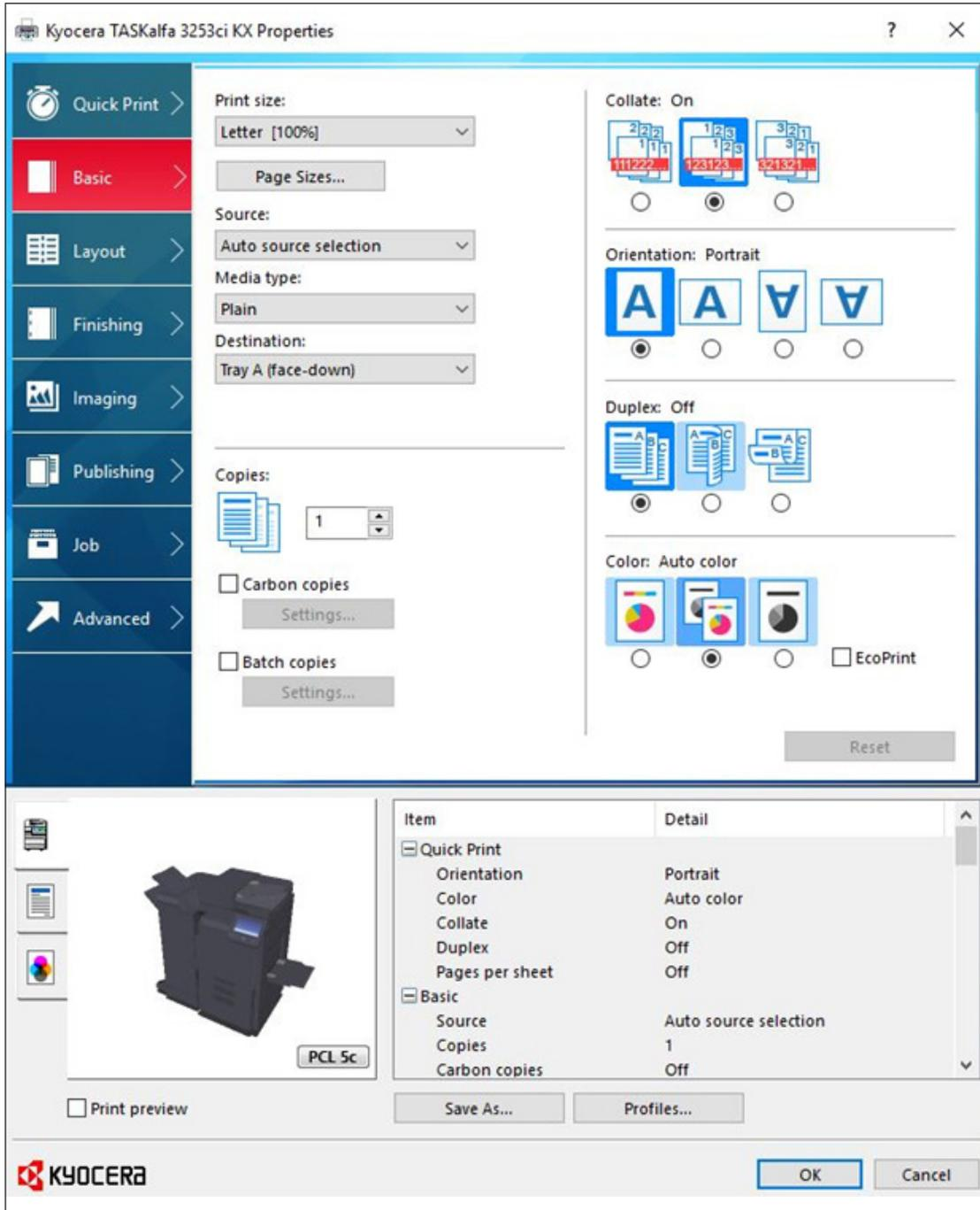
Most typical print job settings are selectable from the Basic tab, including paper type and source, duplex, EcoPrint On/Off, quantity, and collate sets, although finishing selections such as stapling are programmable from the Finishing tab.
