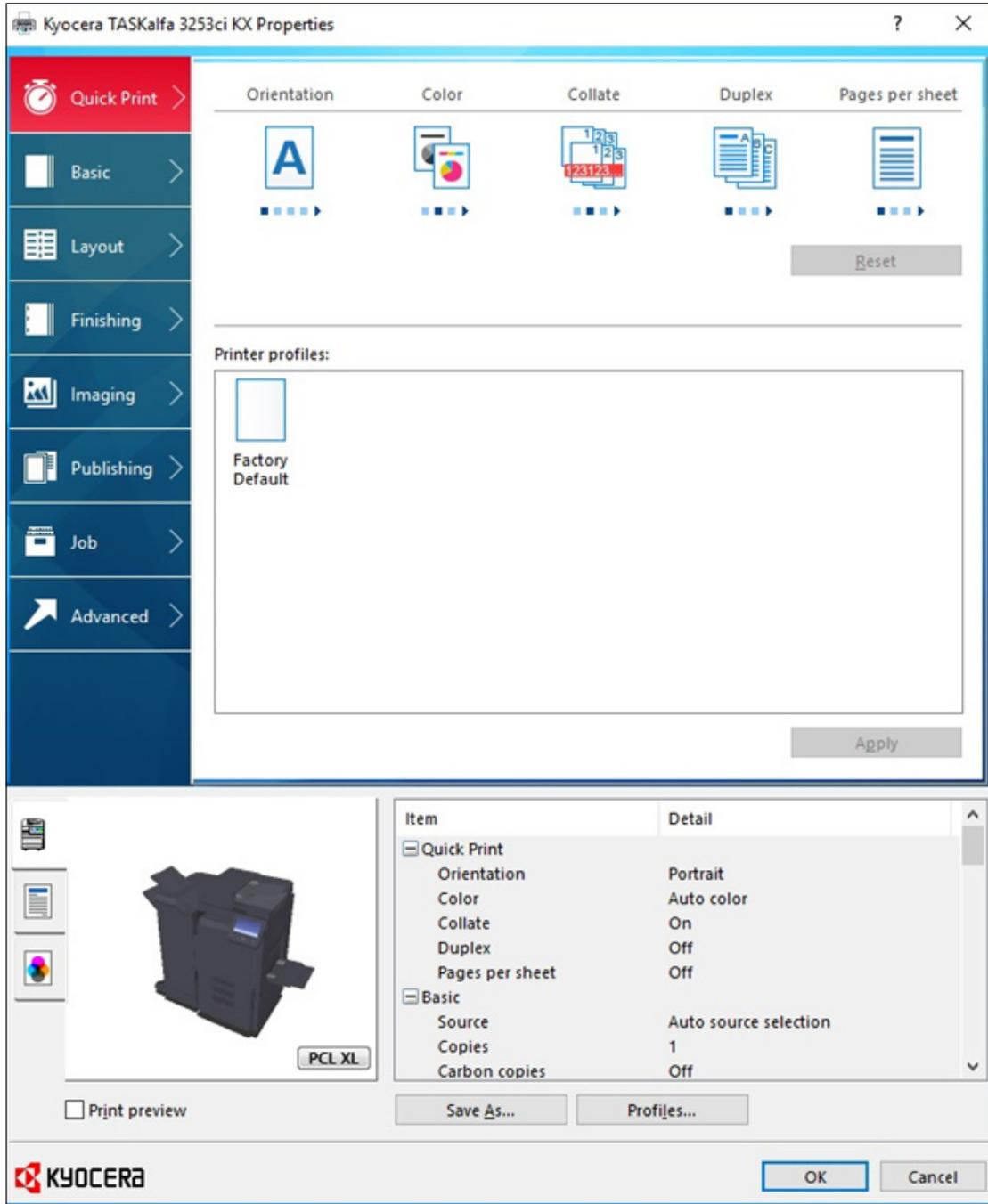
While an entire tab of the driver cannot be customized, users can save custom profiles that are stored as graphical icons via the Quick Print tab to allow programming of complex jobs in one click. Users can click on the Save As button on any of the tabs to save currently selected settings, name the new profile, and add a description for storage on the Quick Print tab.
