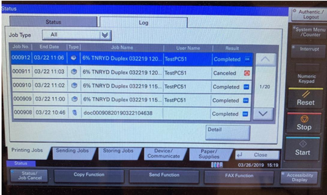
Users can view all print, scan, and copy jobs in a single list, or they can choose to view only specific types of jobs. The number of originals and numbers of sets in a job are listed, as are jobs that are complete and incomplete. The queue displays the total number of sets in a job, but not the time until job completion. Jobs can be promoted to the top or one slot at a time for maximum flexibility. However, jobs cannot be modified beyond quantity.
