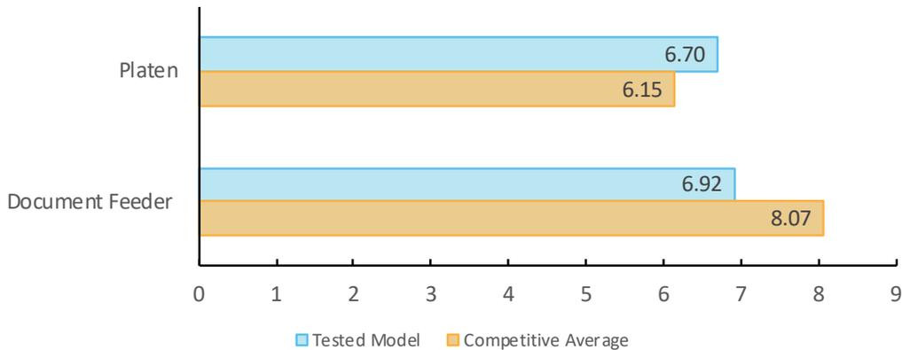
First-copy time is measured as the time it takes for a single copy to completely exit the device when a copy is made from an original placed in the document feeder and on the platen.
