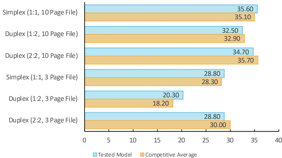
Copy speed is tested using 3-page and 10-page mixed-color and black documents. Buyers Lab obtains the overall speed by averaging the tested speed for each run length (1, 5, 10, and 20 sets).
