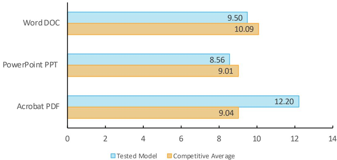
First-print time indicates the time it took to process the image and deliver a single-page test document to the output tray. The unit was tested using the PCL driver.
