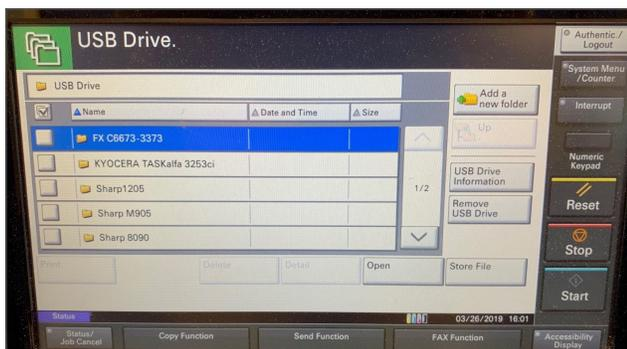
The print from USB menu is automatically populated, with support for PDF, JPEG, and TIFF formats. Users can also change settings for quantity, simplex/duplex, and paper size and source. Users can also navigate and print from sub-folders. However, file preview did not function.
