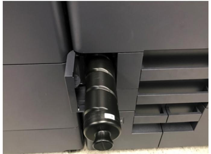
The process for replacing toner is simple and clean. Only when the container is empty will the device notify the user to open the front panel and make the replacement, helping to prevent premature replacement of toner. Guidance at the control panel is extensive and includes text, graphics, animation, and video.
