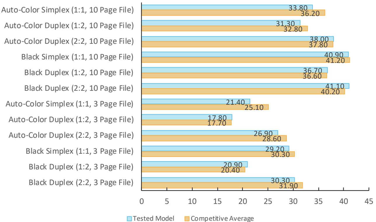
Copy speed is tested using 3-page and 10-page mixed-color and black documents. Buyers Lab obtains the overall speed by averaging the tested speed for each run length (1, 5 and 10 sets).
