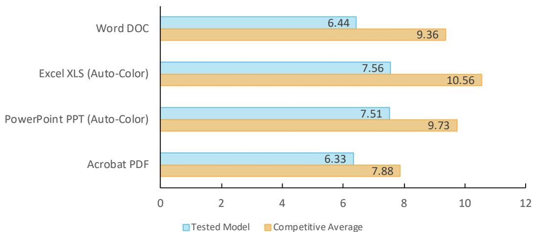
First-print time indicates the time it took to process the image and deliver a single-page test document to the output tray. The unit was tested using the PCL driver.
