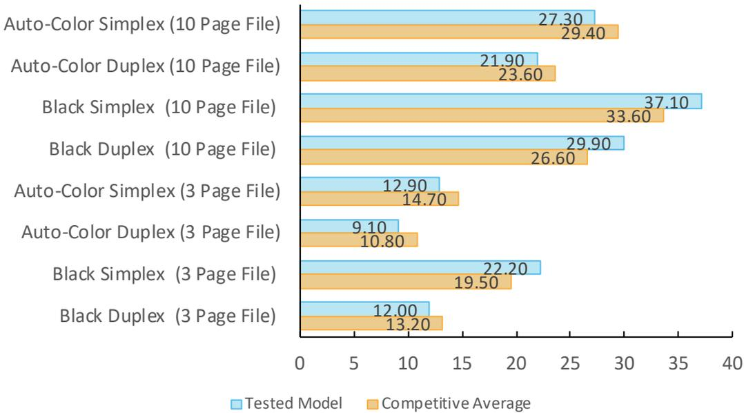
Single-set speed is tested using Buyers Lab's proprietary 3-page and 10-page testing documents. The unit was tested using the PCL driver.
