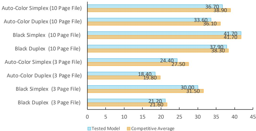
Speed is tested using Buyers Lab's proprietary 3-page and 10-page testing documents. Buyers Lab obtains the overall speed by averaging the tested speed for each run length (1, 5 and 10 sets). The unit was tested using the PCL driver.
