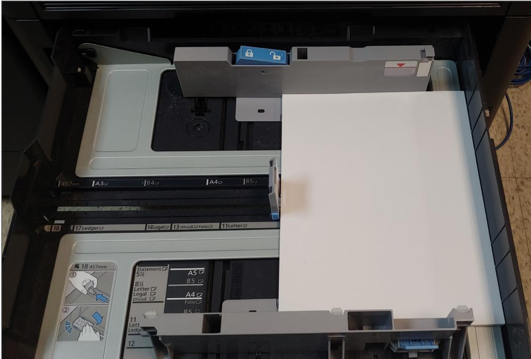
Both length and width guides slide in sync when adjusting paper size in the drawers and have blue locking tabs for easy view. The drawers also feature easy-to-see limit indicators, and soft close once paper is loaded.
