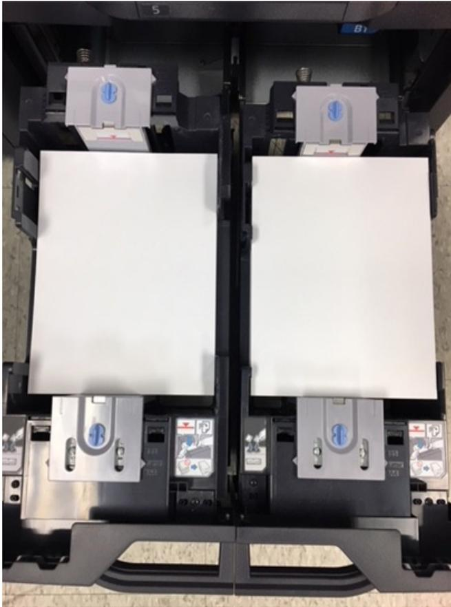
Both length and width guides slide in sync when adjusting paper size in the drawers. In addition, stickers available on side-to-side guides are easy to read and break down different height limits from standard paper to envelope height. Plus, the soft close drawers make for no slamming of cassettes.
