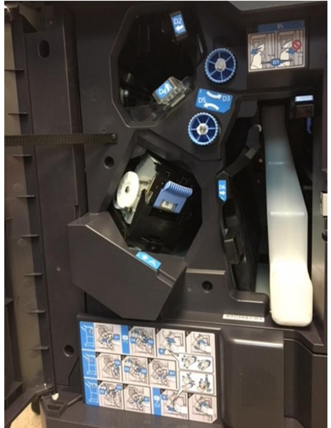
Dynamic, step-by-step instructions are provided for clearing misfeeds (finisher pictured) and include text, graphics, and animation. All misfeed areas allow for easy access, and all user access handles are clearly marked blue.
